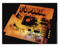
this card does is calibrate the Toaster within 10 Hz of the Toaster's Crystal Oscillator, successfully solving most problems associated with "Will Not Genlock" and "Toaster Not Responding" messages. It also checks the Amiga's power supply (with the ability to check a PC power supply too) and comes with an instructional video tape.
